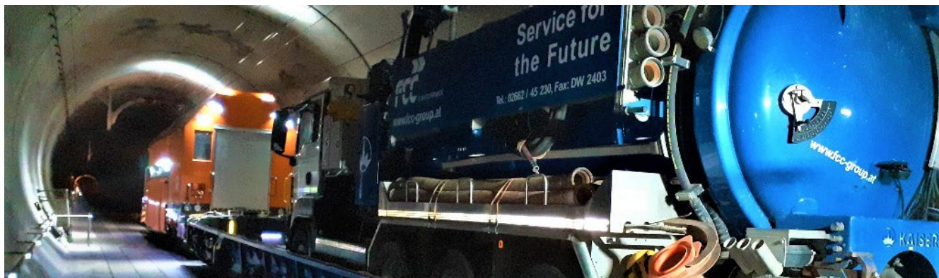
Drainage system cleaning tank.
