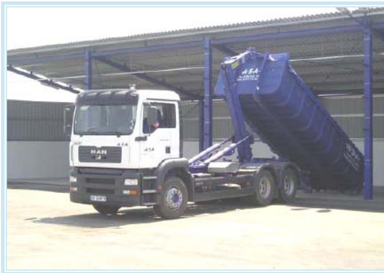
Container-loading vehicle for bulky waste
