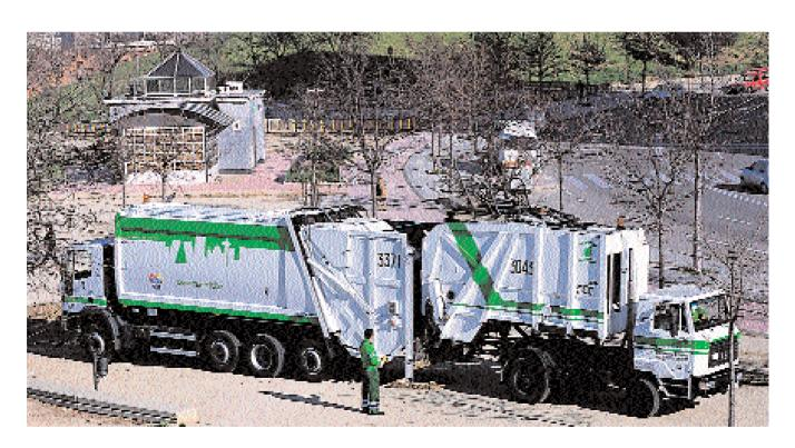
axles is very short in order to obtain a minimum turning radius, 27 m³ of body volume and a maximum length of 10.5 m.
