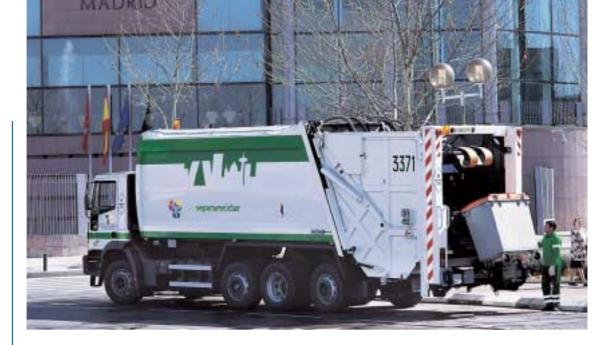
containers and other residential waste. The trash is unloaded through two completely independent rear doors to impede the different types of trash from mixing together. The lower compartment is emptied first, while the upper compartment remains closed, after which the upper compartment is emptied.
