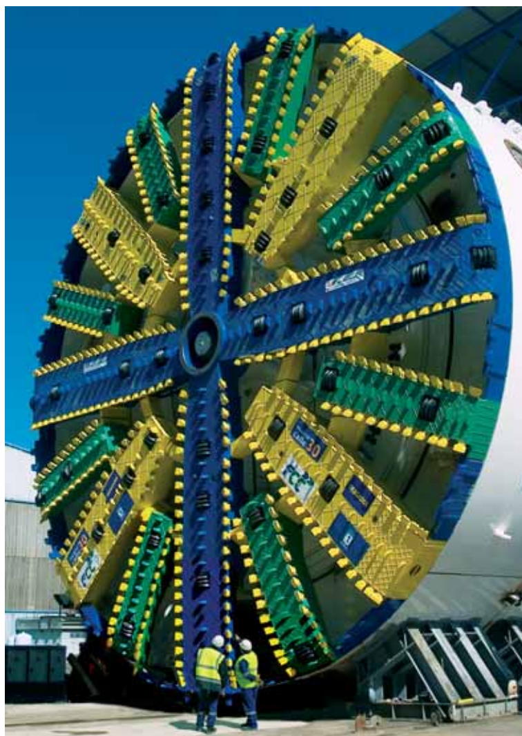
TBM for enlarging the M-30. Madrid
