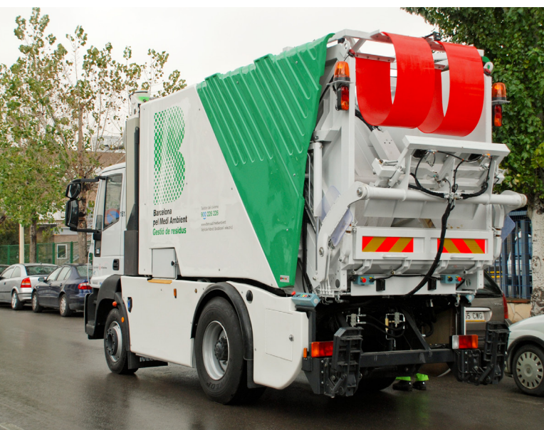
Electric-hybrid vehicle for urban solid waste collection, Barcelona.
