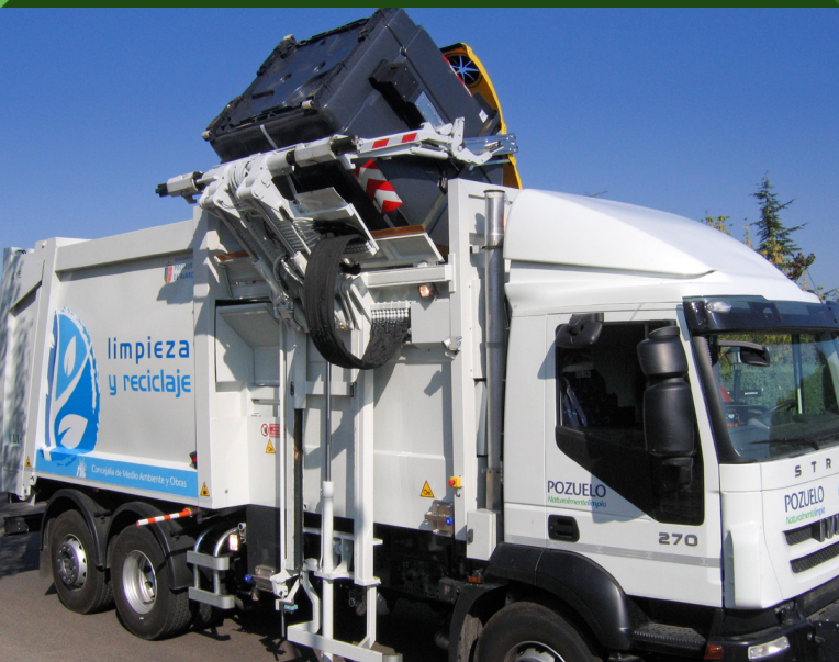
Side loading collection vehicle.
